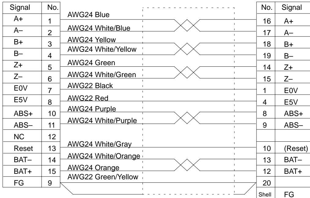
Cable: AWG22 × 3C + AWG24 × 6P
