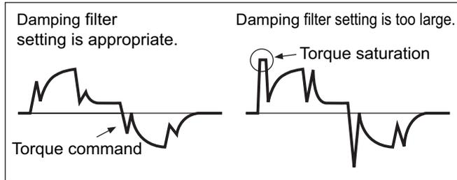
When setting the damping frequencies, reduce the setting if the torque become saturated and increase the setting to make operation faster. Normally 0 is set.
