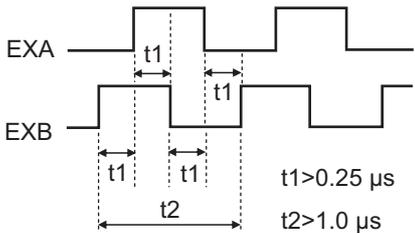
\*1 Connect external encoder signals to the serial interface (+EXS/-EXS) or 90° phase difference inputs according to the encoder type.
