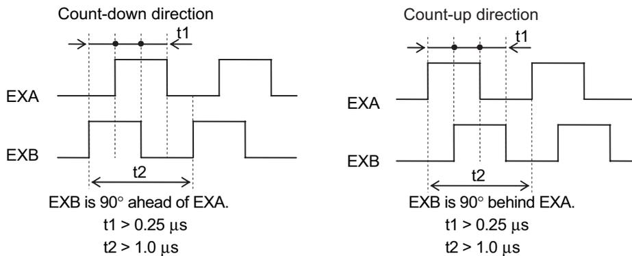
\*3 For the external encoder connection direction, set the direction so that count-up occurs when the motor shaft is rotating counterclockwise, and count-down occurs when the motor shaft is rotating clockwise. If the connection direction cannot be selected due to installation conditions or any other reason, the count direction can be reversed using External Feedback Pulse Direction Switching (3326 hex).
