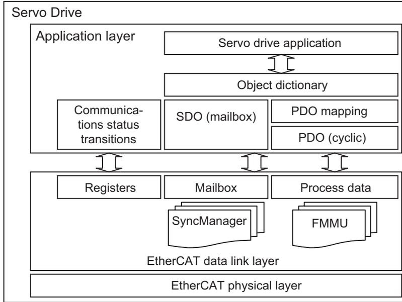
Normally, multiple protocols can be transmitted using EtherCAT. The IEC 61800-7 (CiA 402) drive profile is used for OMNUC G5-series Servo Drives with Built-in EtherCAT Communications.
