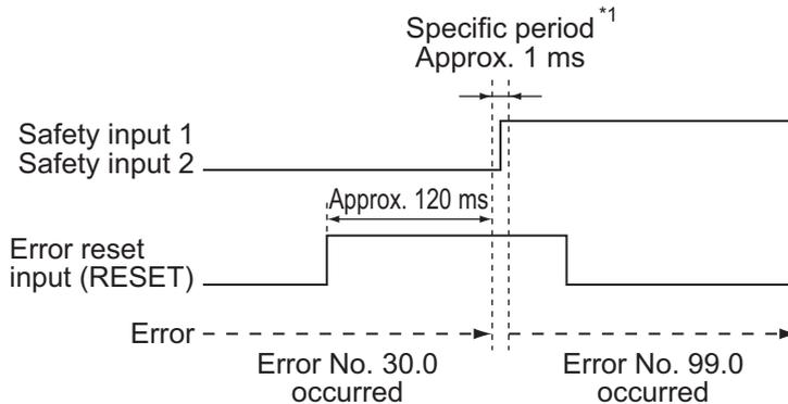
\*1 Error No. 99.0 will occur if at least one of the input photocouplers for safety inputs 1 and 2 is turned from OFF to ON.
