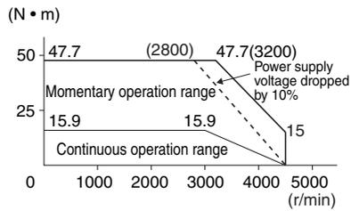
Note: The continuous operation range is the range in which continuous operation is possible. Continuous operation at the maximum speed is also possible. However, doing so will reduce the output torque.
