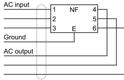
♦ Use twisted-pair cables for the power supply cables, or bind the cables.
