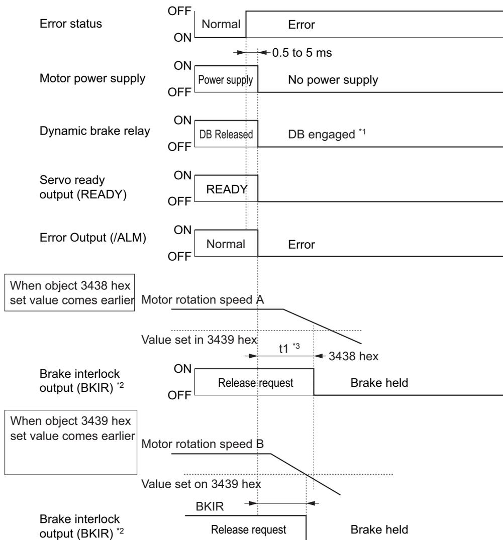
\*1. The operation of the dynamic brake when there is an error depends on the setting of the Fault reaction option code (605E hex).
