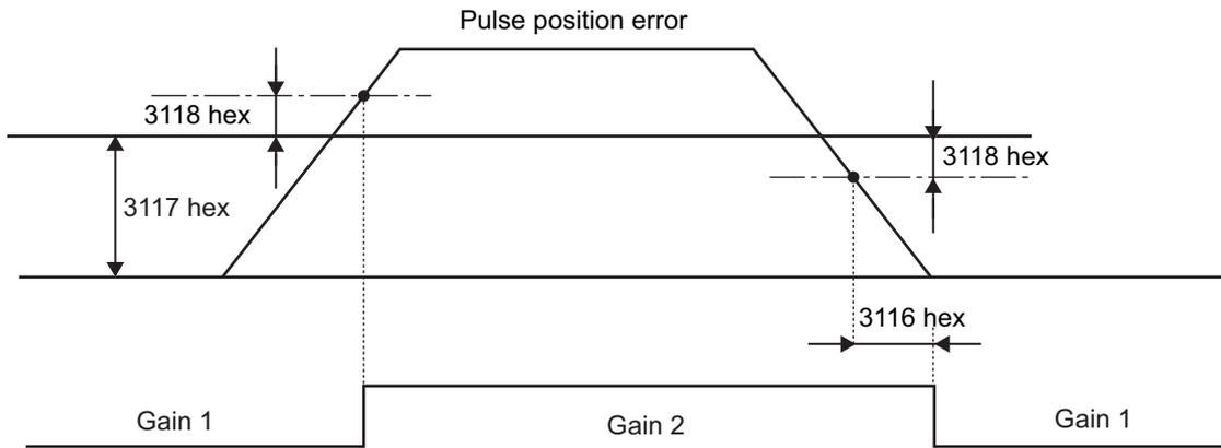
**Gain Switching Mode = 7: Switching by Whether There Is a Position Command**
