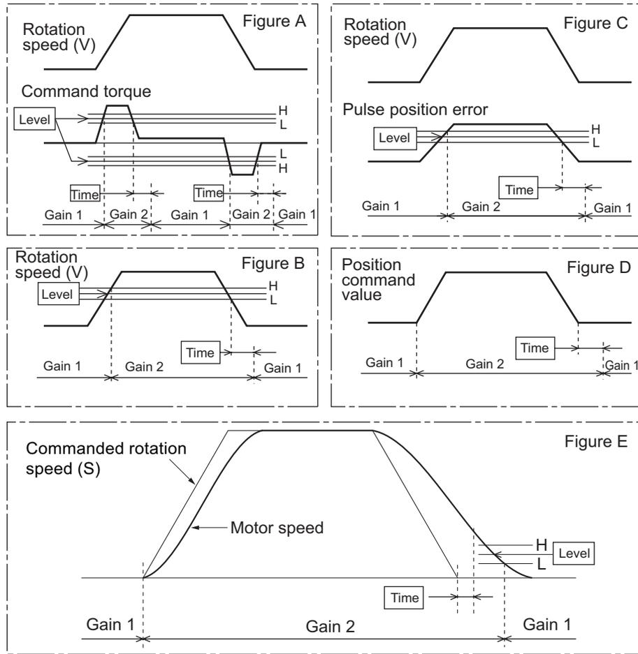
**Diagrams of Gain Switching Setting**
