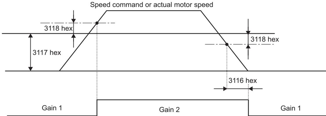
Note: The "speed command" is the Motor Control Effort (401A hex) [r/min].
