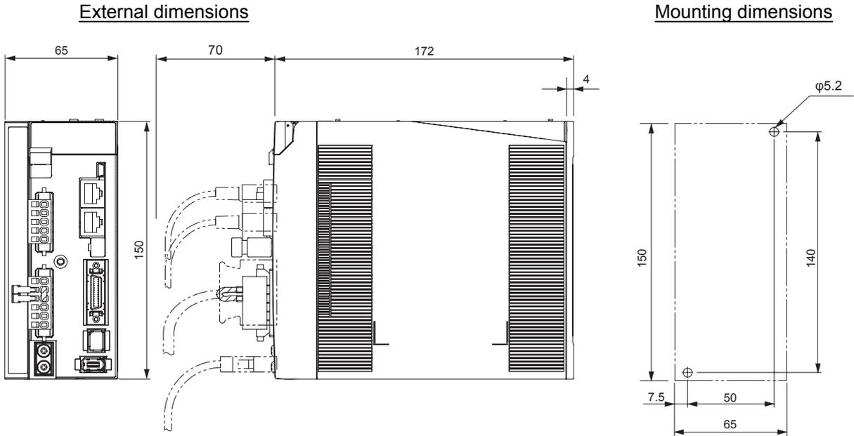
**Front Mounting (Using Front Mounting Brackets)**
