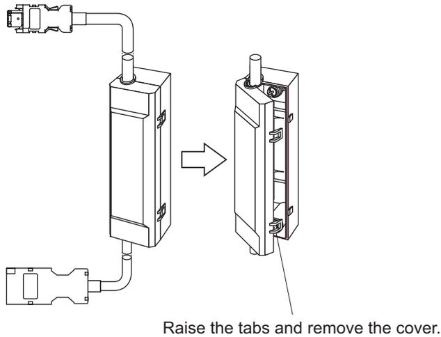
3. Put the Battery Unit into the battery box.
