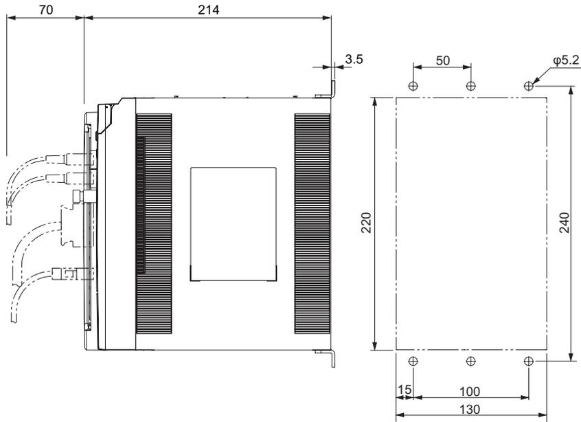
**Front Mounting (Using Front Mounting Brackets)**
