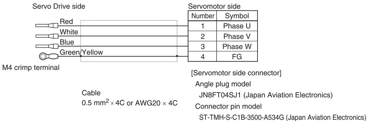
Note: For servomotors with brake a separate cable R88A-CAKA□□□BR-E is needed.
