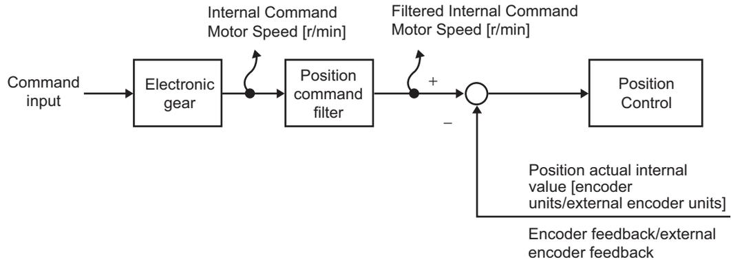
\*2. The position error is calculated for the command input after processing for the position command filter. The pulse position error or fully-closed position error is reversely converted to command units for application. The pulse position error or fully-closed error is the error for the position control input.
