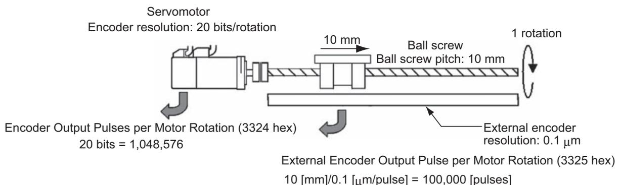
$$\frac{\text{Object 3324 hex}}{\text{Object 3325 hex}} = \frac{\text{Encoder resolution per motor rotation [pulses]}}{\text{External encoder resolution per motor rotation [pulses]}} = \frac{1048576}{100000}$$
