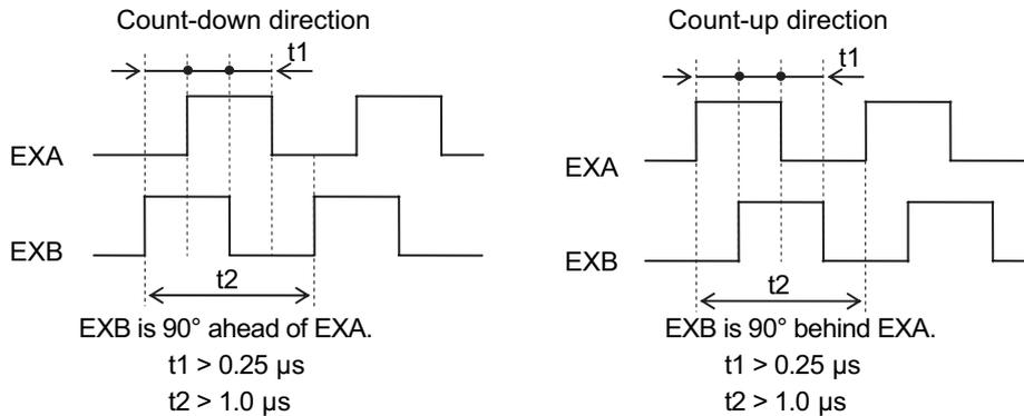
\*3 For the external encoder connection direction, set the direction so that count-up occurs when the motor shaft is rotating in the CCW direction, and count-down occurs when the motor shaft is rotating in the CW direction. If the connection direction cannot be selected due to installation conditions, the count direction can be reversed using External Feedback Pulse Direction Switching (3326 hex).
