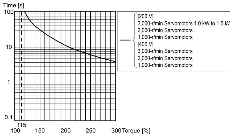
When the torque command = 0, and a constant torque command is continuously applied after 3 or more times the overload time constant has elapsed, the overload time  $t$  [s] is
