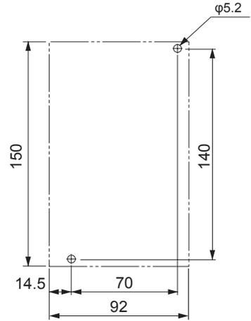
**Front Mounting (Using Front Mounting Brackets)**
