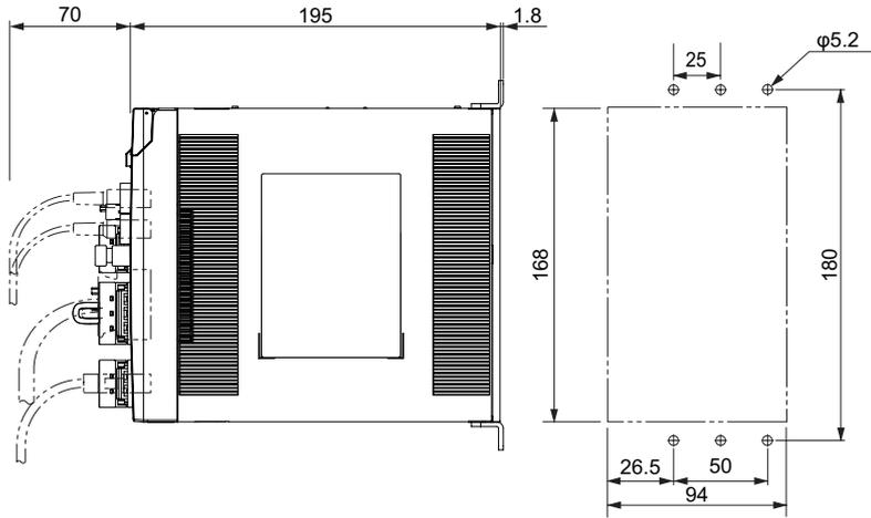
Front Mounting (Using Front Mounting Brackets)
