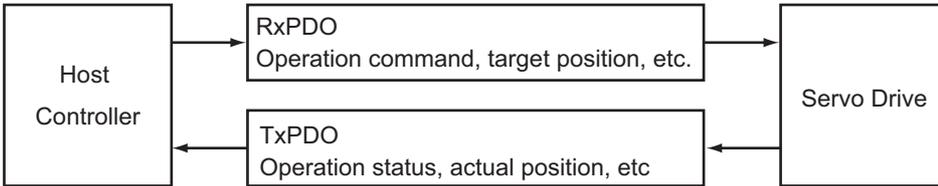
The EtherCAT application layer can hold multiple objects to enable transferring Servo Drive process data. The contents of the process data are described in the PDO Mapping object and the Sync manager PDO assignment object.
