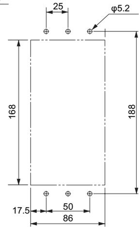
Front Mounting (Using Front Mounting Brackets)
