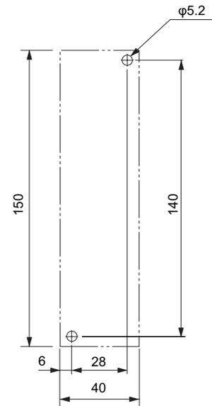
Front Mounting (Using Front Mounting Brackets)
