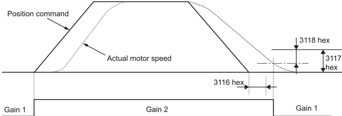
Note: Whether there is a position command is determined by changes in the Target position (607A hex).
