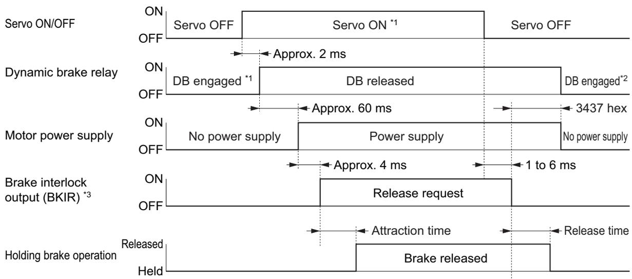
\*1. The servo does not turn ON until the motor rotation speed drops to approx. 30 r/min or below.
