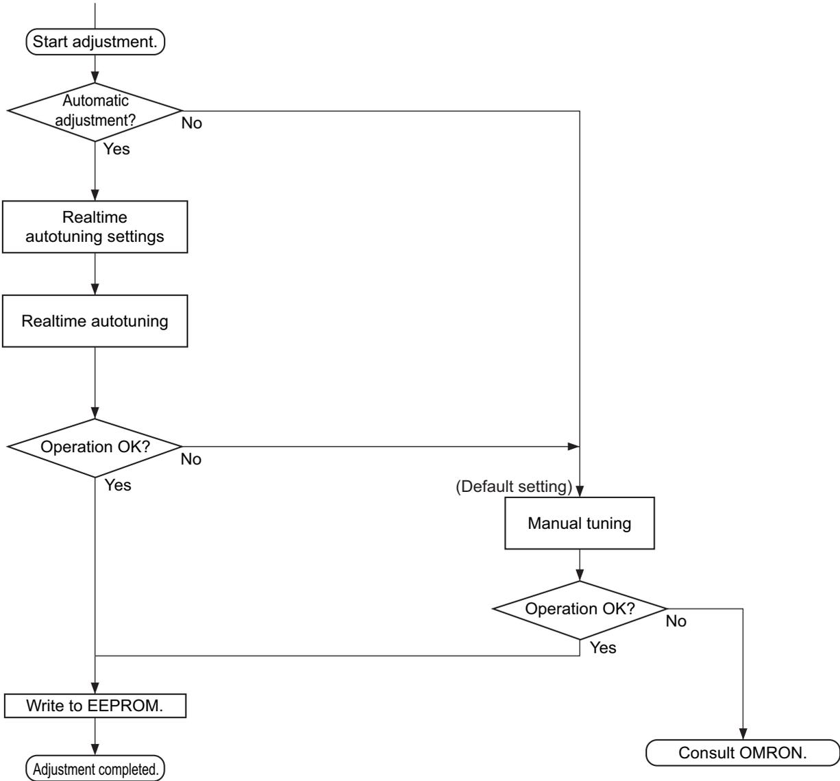
**Gain Adjustment and Machine Rigidity**
