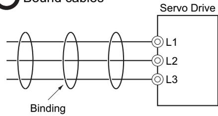
♦ Separate power supply lines and signal lines when wiring.
