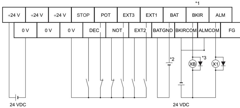
\*1. Assign the brake interlock output (BKIR) to pin CN1-1.
