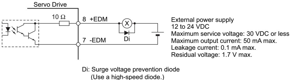
Note: When driving a relay directly with an output signal, always insert a diode as shown in the above figure.
