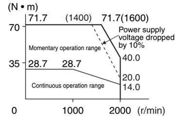
Note: The continuous operation range is the range in which continuous operation is possible. Continuous operation at the maximum speed is also possible. However, doing so will reduce the output torque.
