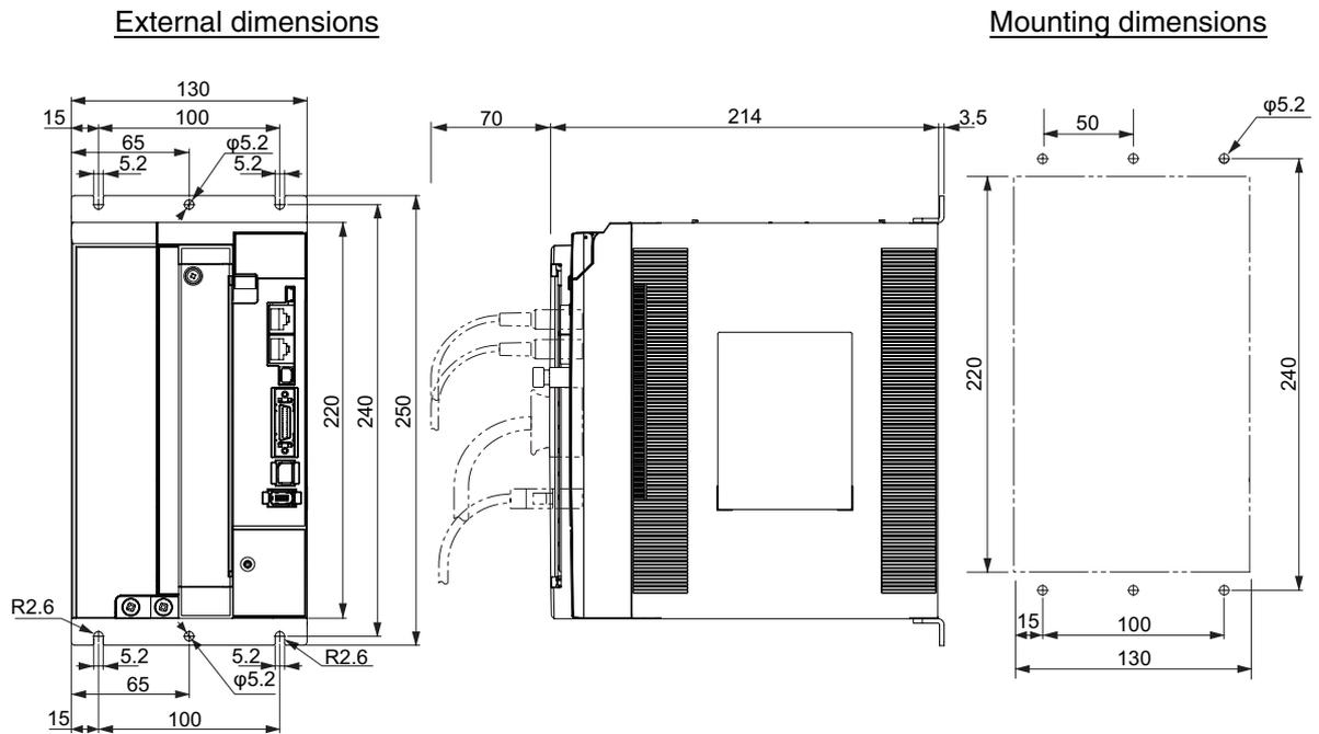
**Front Mounting (Using Front Mounting Brackets)**
