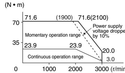
Note: The continuous operation range is the range in which continuous operation is possible. Continuous operation at the maximum speed is also possible. However, doing so will reduce the output torque.
