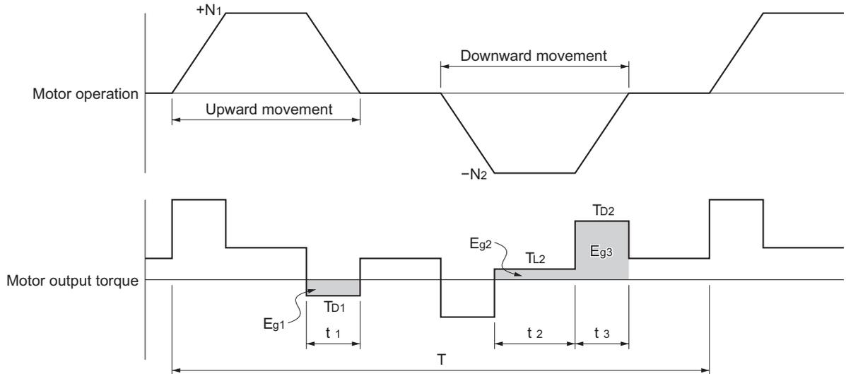
• In the output torque graph, acceleration in the forward direction (rising) is shown as positive, and acceleration in the reverse direction (falling) is shown as negative.
